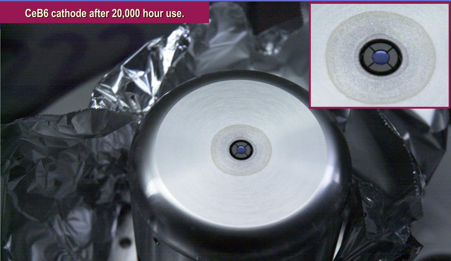
It was found the cathode surface became concave of 0.2 mm deep from the initial flat surface. It corresponds to evaporation speed of 10 nm/hour (  $10 \text{ nm/h} \times 20,000 \text{ h} = 200 \text{ micron-meter}$  ) Concave geometry made beam slightly focusing, but did not break emittance. Electron microscope study showed (1) Surface is fairly smooth, (2) covered by carbon contamination (lowered electron emission).
