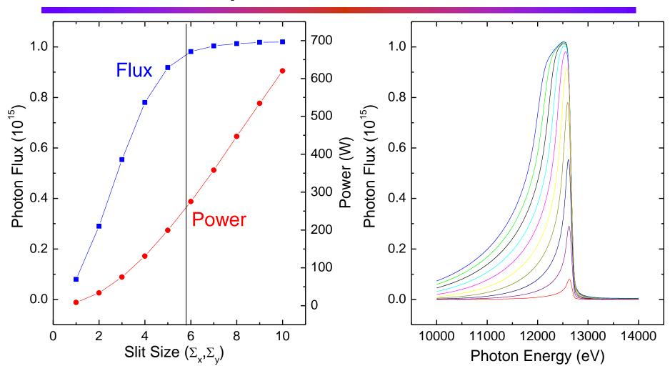
Too wide aperture results in broader bandwidth and unwanted heat load.
