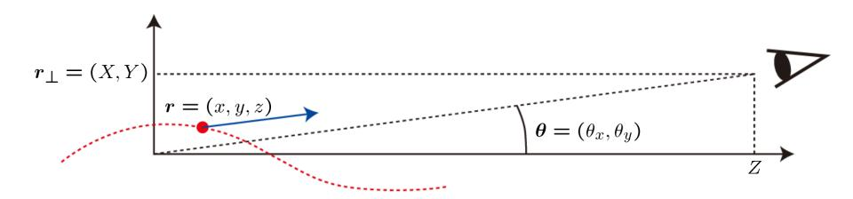
SR emitted by an electron moving at  $\mathbf{r} = (x, y, z)$ Observation of SR at  $\mathbf{R} = (X, Y, Z)$
