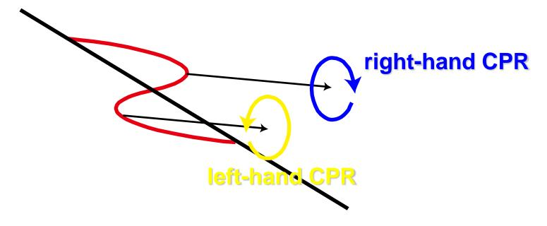
EMPW is a special wiggler to utilize CPR by introducing a vertical motion.
