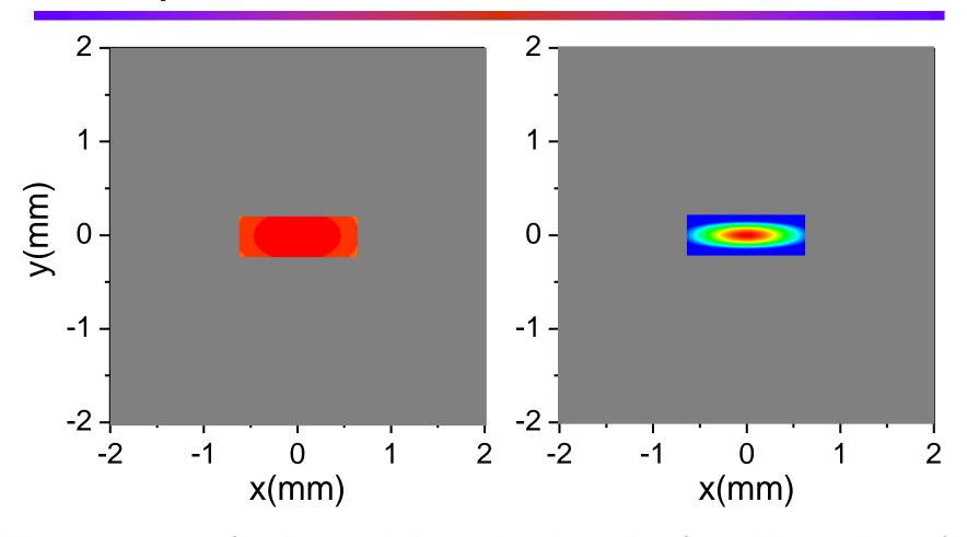
The power profile is much broader than the flux. Extraction of SR with an appropriate slit significantly reduces the heat load.
