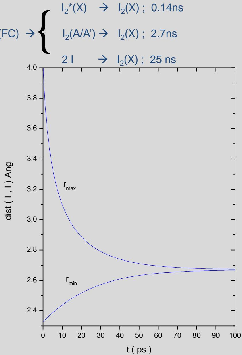
Recombination of I<sub>2</sub> in CCl<sub>4</sub>(1:500) probed with 100 ps resolution
