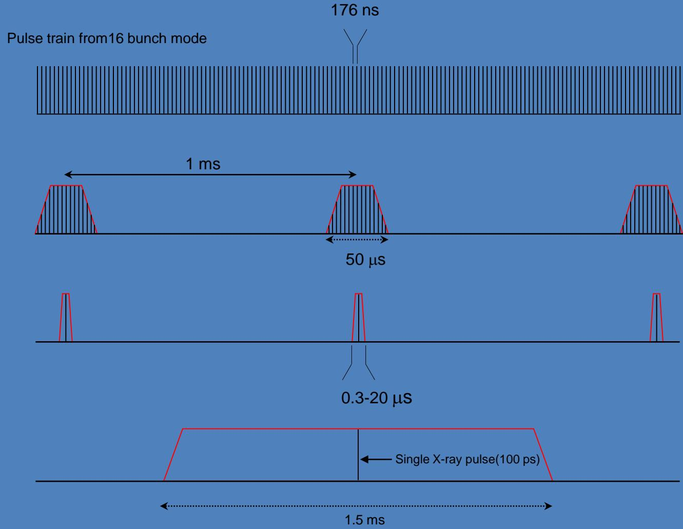
Pulse lengths: 50 ps to 50 us, Pulse frequency: 0-1000 Hz
