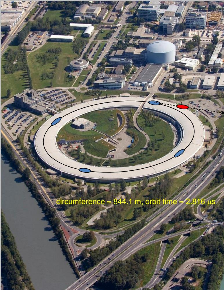
Synchrotron emits intense 100 ps X-ray pulses with up to  $\sim 10^{10}$  ph per pulse
