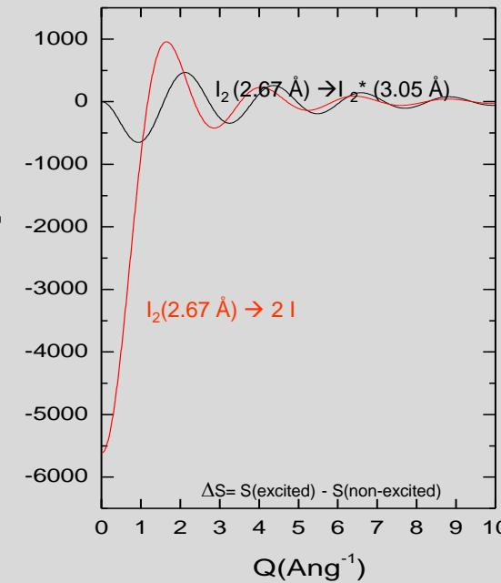
Fourier transform of  $\Delta S(q, \tau)$  is a measure of the change in radial electron density
